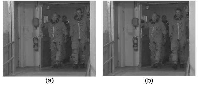
Figure 4: Interpolated frames in the presence of flashlight: (a) before pre-processing (21.56dB), and (b) after pre-processing (28.81dB).
